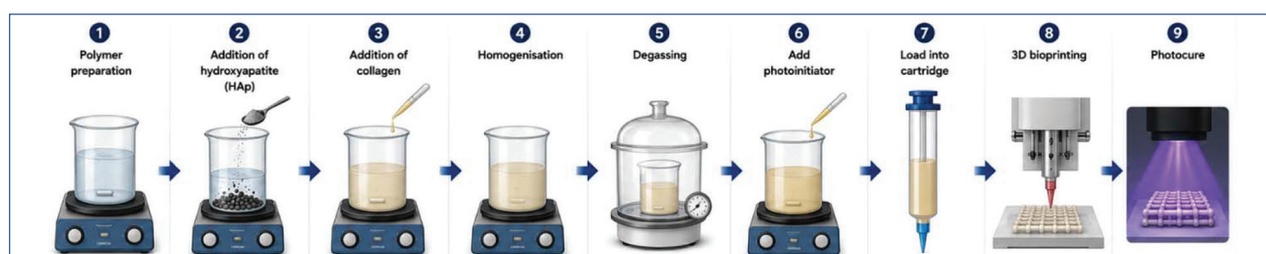
[Table/Fig-1]: Schematic representation of Biomaterial Ink (BI) development and 3d bioprinting process.
